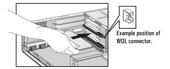
6 Connect the Remote Wake-Up cable to the connector on the card and to connector on the system board or backplane.
